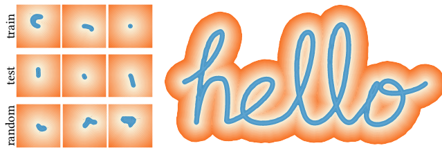
Figure 14: We train a neural swept volume network with a circle sweep shape on a set of handwriting paths obtained from [Marti and Bunke 2002], visualized on the left. On the right, we demonstrate how our method is able to produce and generalize an exact SDF of the “hello” that is written by a writer not included in the training data.
