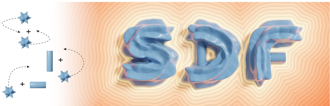
Figure 1: Our method allows for the computation of exact neural SDFs of CSG operations. Here, we train one network to learn the swept volume of a stellated dodecahedron shape, parametric over the control points of the cubic Bézier path it is swept along. Specific swept volumes within this parameter space are then unioned together and with cylinders, resulting in a neural implicit which thanks to our regularization term forms an exact SDF of the word “SDF.”
