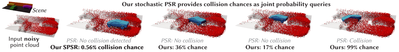
Fig. 20. We can use our statistical formalism to compute statistical quantities like collision chances (bold), unlike traditional PSR (grey).
